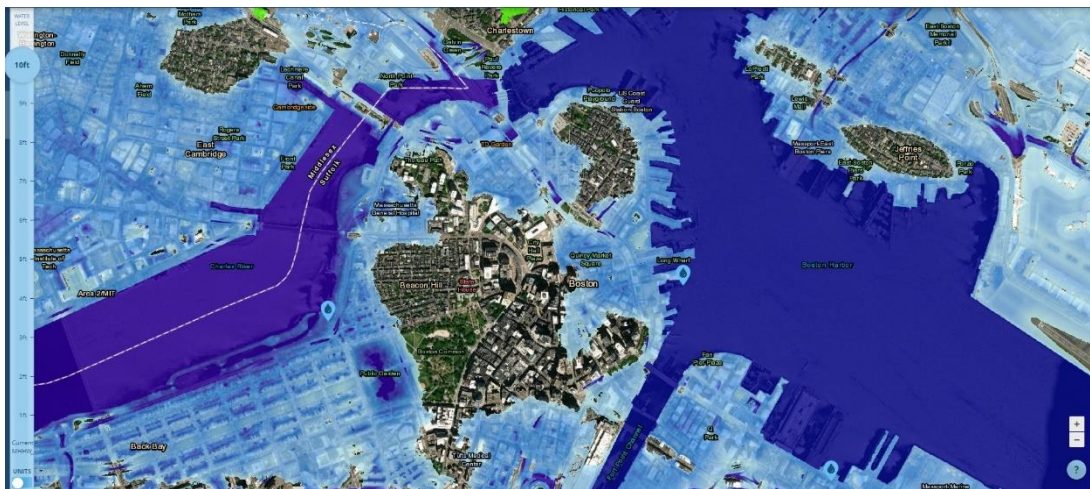
Figure 5. The official National Oceanic and Atmospheric Administration "Sea Level Rise Viewer" for Boston and Cambridge falls four feet short of actual storm surge from Hurricane Sandy, which was 14 feet when it hit New York in 2012. Even at ten feet of storm surge, Boston's infrastructure and access to the capital would be swamped. Public Domain https://coast.noaa.gov/slr/#/layer/slr/10/-7910282.712677894/5215253.588984675/15/satellite/none/0.8/2050/interHigh/midAccretion
